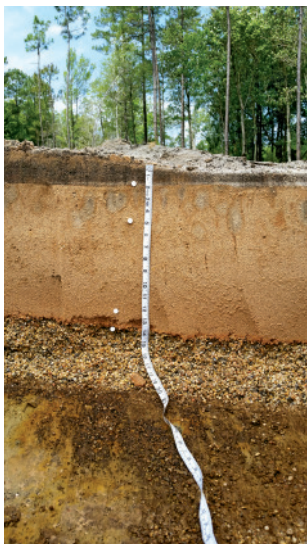
Thin clay band at the interface of sand and gravel (14-inch depth) in a nine-year-old putting green in Mississippi.
