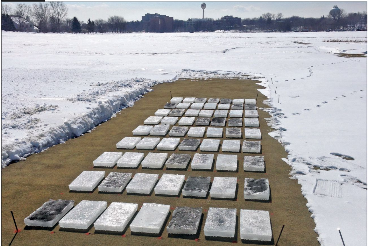
An ice melting study at the University of Minnesota's Turfgrass Research, Outreach and Education Center, conducted this last winter. These manufactured ice blocks were treated with 20 different salt and solar absorption products to evaluate ice melting potential. More detail on this study can be found at: www.turf.umn.edu .
