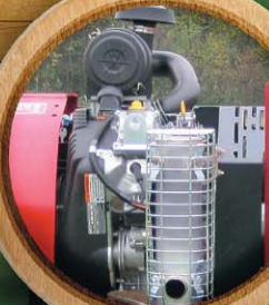
31 hp Briggs and Stratton engine, all wheel drive
