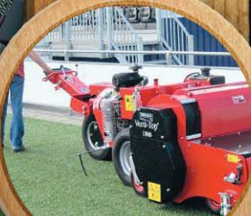
31 hp Briggs and Stratton engine, all wheel drive
