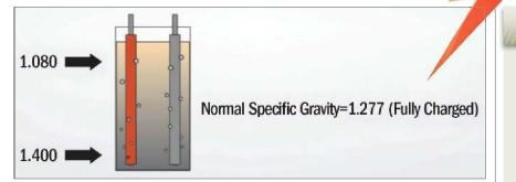
Stratification occurs when denser electrolyte sinks to the bottom of the battery, harming the battery's plates.
