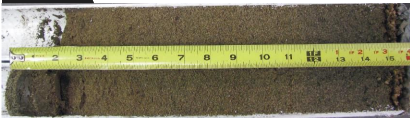
Full profile view of sand-based putting green using a PVC pipe sampling method. Note the oxidized iron layer at the sand/gravel interface (15-inch depth).
