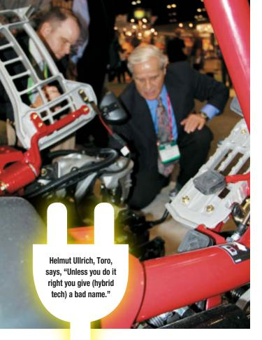
models. The TriFlex Hybrid models feature an all-electric reel drive system that virtually eliminates hydraulic leaks and delivers ample horsepower to handle a broad range of cutting applications. Also, the traction unit is equipped with tool-free, quick change cutting units so it can be converted for spiking, thatching or verticutting in just a few minutes.
