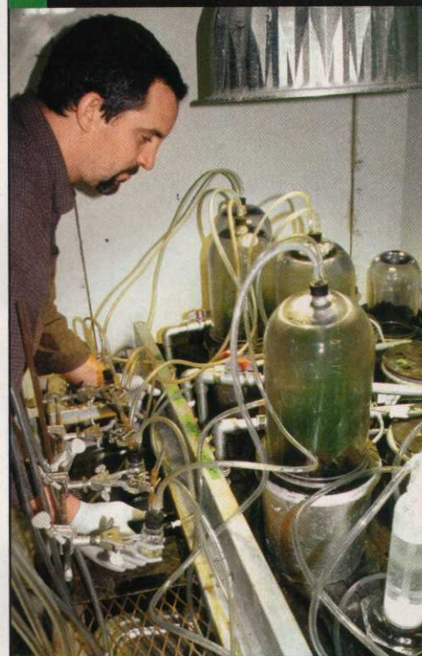
John Bushoven makes adjustments to growth chamber-mounted units for exposing leaves of turfgrass cultures to elevated \text{CO}_2 concentrations or ^{14}\text{CO}_2 .
