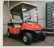
double rack-and-pinion steering, limited slip differential, a cushioned steering wheel and energy-transfer bumpers, among other features, E-Z-GO's new RXV is inching closer to its electric car cousin.
