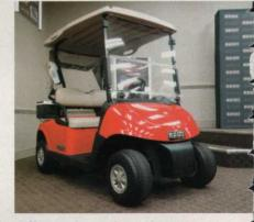
double rack-and-pinion steering, limited slip differential, a cushioned steering wheel and energy-transfer bumpers, among other features, E-Z-GO's new RXV is inching closer to its electric car cousin.
