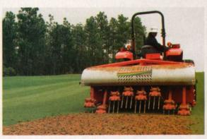
among the fastest, while a hydraulic top-link allows users to adjust aeration depth on the fly during transport or while in use. The respective 60- or 80-in. swaths can core up to 65,000 and 98,000 square feet per hour, making the PerformAire aerators adaptable to any job at any depth while promoting healthier, faster-healing turf.
