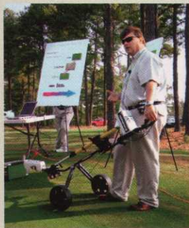
Richard Rees, Ph.D., demonstrates the NTech GreenSeeker, which translates light reflection into a vegetative index to determine turf health.
