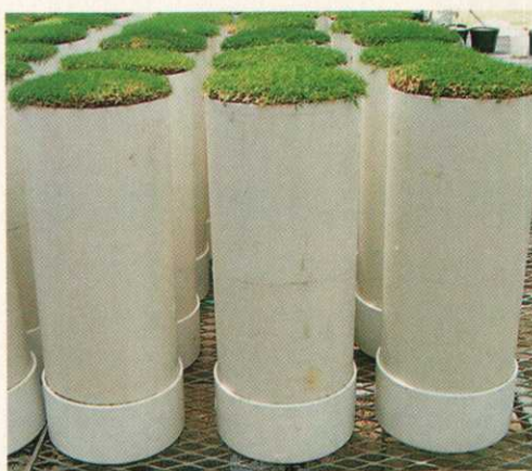
Lysimeters built to USGA specifications are used for greenhouse experimental units.
