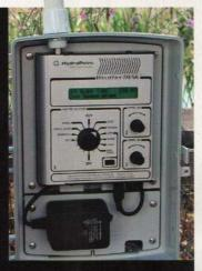
and slope and calculates how to apply the right amount of water at the right time. The wireless ET (Evapotranspiration) Everywhere Data Service delivers daily weather updates to each controller, allowing the scheduling engine to adjust watering automatically based on actual plant needs.
