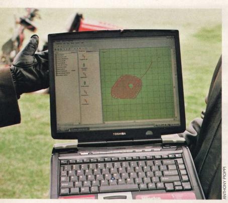
This is how the computer screen appears when the unmanned mower is in use. The circular green spot within the red spot is the mower. Wagner envisions a chaperone watching over up to four machines simultaneously, acting as the mother goose to the flock of mowers.
