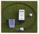
which provides superintendents with thorough soil moisture content, salinity and temperature information. The Hydra Probe system also helps course personnel manage optimal watering and fertilization effectiveness.
