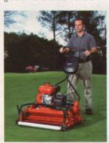
feature greens-hugging, floating head reels. Suspended from the chassis, the floating reel of the Tournament Cut mower moves horizontally, vertically and from side-to-side to eliminate scalping severely undulating greens. For more information, contact 704-504-6600, www.jacobsen.com or CIRCLE NO. 203
