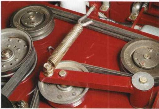
*Inspect spindles and pulleys, paying particular attention to bearings, belt conditions and tensions.*
