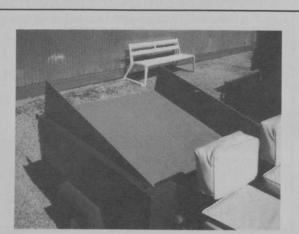
With the cost of golf course maintenance vehicles over \$4,000, here is an idea one might try to help protect the rear box on the vehicle. At the Golden Horseshoe golf course, the mechanic built thin wooden liners that could be placed inside the rear box.
