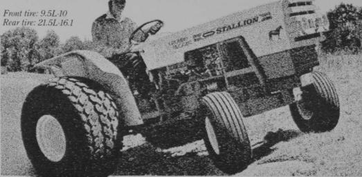
Satoh satisfaction starts with the Stallion Ground Hugger's dependable, smooth-running 38hp water-cooled Diesel engine. With nine forward speeds (three reverse) and dualspeed live PTO (540 and 1,000 rpm), the cost-efficient Stallion Ground Hugger is ideal for hilly terrain uses such as municipal park maintenance and golf course grooming.
