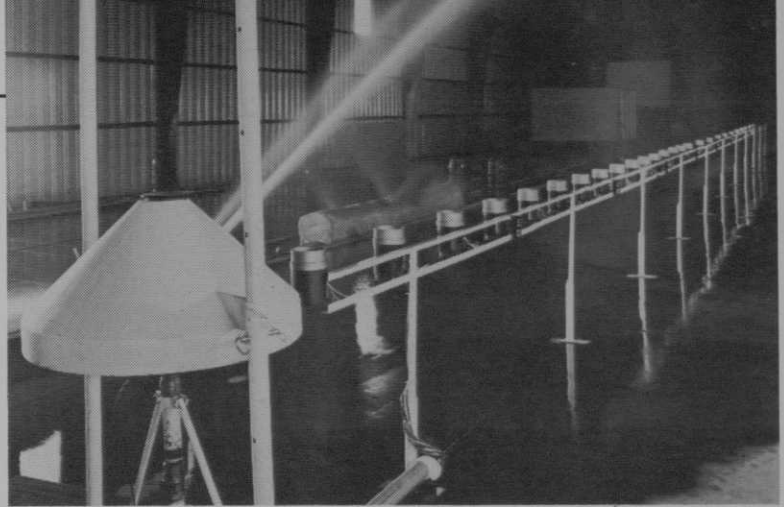
Sprinkler tests are conducted indoors under no-wind conditions to insure proper and concise recording of performance data. Digital counters record the amount of water in the catchments.
