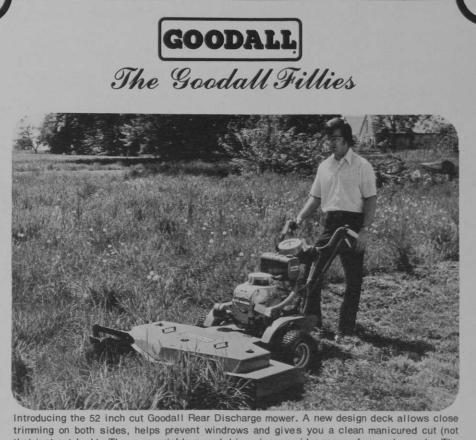
that just-cut look). The new variable speed drive gives a wider range of ground speeds. The 3 gallon fuel tank and Hi-Way front caster wheels are standard equipment. This new mower is designed for fine lawns and rough areas. The finger tip control gives the same easy handling and hillside stability and maneuverability as the other Goodall Self-Propelled models. Also available is a new 36 inch rear discharge mower.
