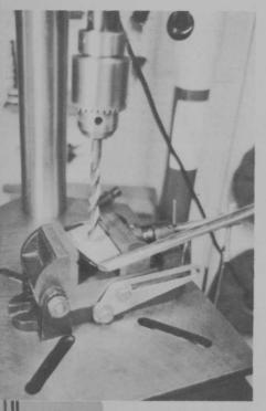
Correcting the lie in clubs is another important part of re-pair. To demonstrate this, get an old 4, 5 or 6 iron and by using a drill press (top) bore a 3/ inch diameter hole in the approximate center of the face. At bottom, an old shaft is pushed into the hole. The angle of the protruding shaft helps indicate the lie of the club and show customers the importance of the proper lie.
