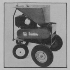
VANDERMOLEN CORP. adds a 12hp heavy-duty chipper to its 1973 Diadem Brush Chipper Line, which offers the highest hp available on small brush chippers. The unit features the Diadem single casting rotor, which chops branches of up to three inches in diameter into small chips, ideal for mulch and compact bagging. The chipper is available as a skid or wheeled model with four pneumatic tires and roller bearing wheels.
