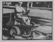
THE TORO COMPANY introduces the Groundsmaster 72 riding rotary mower, first of a new "silent breed" without belts or chains. It can be easily converted into a snow-thrower or sweeper. It has a 72-inch cut, modern styling, electric start, rear-wheel steering, eight-hour fuel capacity, low center of gravity, short-turning radius and quick forward-reverse. Circle No. 102 on reader service card
