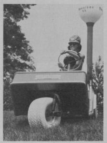
THE FIRESTONE TIRE & RUBBER COMPANY introduces a new cordless cast tire for golf cars in white, yellow, red and blue as well as black. The cast tire, still in the experimental stage, was made possible through the development at Firestone of a rubber so strong that no body-reinforcing materials are needed. The color goes all of the way through the tire. A colored liquid rubber is poured into a mold and after the material sets, the tire is removed.
