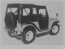
SUZUKI OF SAN DIEGO, United States distributor for the Suzuki vehicle line, announces a swing-away tire carrier on its 1972 models of the Brute IV four-wheel drive. The new tire carrier is a time and trouble saver, according to the company, and has a streamlined appearance. Other features of the Brute IV include dual-stroke action/engine, and an oil injection system. The vehicle gets up to 30 miles per gallon. Limited dealerships are available. Girde No. 102 on reoder service cord
