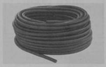
HANCOR, INC., makes Cor-Flow twoinch flexible drainage tubing. The perforated pipe can be laid in any direction without intermediate fittings and can be cut to any length with a knife. The tubing is acid, alkali and frost-resistant and light in weight (a standard 500-foot roll weighs 68 pounds) for easy transportation. Couplers, end caps and tees are supplied. Pipe also comes unperforated. Various diameters are offered, perforated and unperforated. Circle No. 104 on reeder service card
