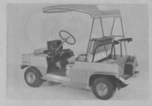
FM stereo, radio and tape deck, black and white TV and a built-in bar. Westinghouse also has the three-wheel *Model 437* and fourwheel *Model 436-E* golf cars. The allsteel constructed electric golf cars feature a 4½ hp traction-rated Westinghouse electric motor.
