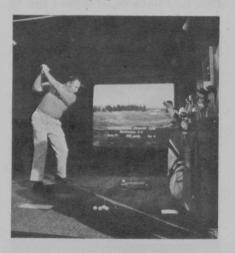
players hitting into a 100-square foot nylon motion-picture screen. A computer calculates the velocity and direction of the ball and advances the filmstrip to the spot on the fairway, rough or hazard where your ball would have landed. Yards driven and the number of yards remaining to the green appear on the screen with each shot. Suggested retail price of *Golfomat* is \$10,000.
