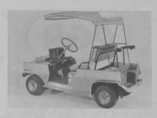
FM stereo, radio and tape deck, black and white TV and a built-in bar. Westinghouse also has the three-wheel *Model 437* and four-wheel *Model 436-E* golf cars. The all-steel constructed electric golf cars feature a 4½ hp traction-rated Westinghouse electric motor.
