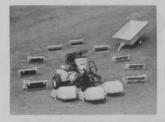
agement System, capable of greens cutting, tee and collar mowing, spiking and verti-cutting. The self-propelled unit can be changed from one operation to another in a few minutes, according to the company. The cutting units are driven by flexible cables, thereby eliminating the possibility of greens damage due to hydraulic hose ruptures.
