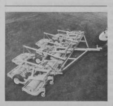
Roseman Mower Corp. introduces an 11-gang hydraulic lift-type mower. Cutting width is 24 feet or about 30 inches per unit. Height of cut is about one-half to three inches. The mower can be used with any utility-type tractor equipped with a hydraulic system.
