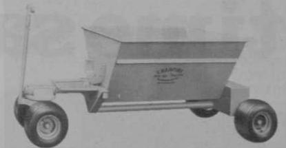
**The Champion Company** offers three models in its *Doo-All Trailer* line. *Roll-Dump* hoppers, available in one-cubic-yard and two-cubic-yard capacities, are also featured on two models. The third model will show the small chassis with the interchangeable flat bed in place. All units feature *Terra-Tires*. The two-cubic-yard chassis has a new square tongue for added strength for sharp turns under heavy load.
