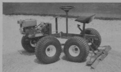
**Stanley Clarke Equipment Company, Inc.**, introduces the *Trap-master* mechanical sand trap rake. One man operating the rake can maintain over 40 sand traps in four hours, according to the company. The rake teeth scarify the trap and the drag plates float out to smooth and finish the trap surface. Stanley Clarke will introduce also several "revolutionary new products."
