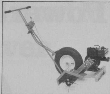
*Edger*. The edger has tempered spring wire tines for all types of grasses. The tines are pivot-mounted and run in reverse direction for fine cutting and so the cut material is thrown ahead and to the side. A depth control allows adjustment for sand traps that are level with the surrounding turf or for traps with high bunkers.
