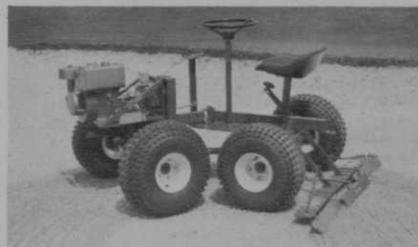
**Stanley Clarke Equipment Company, Inc.**, introduces the *Trap-master* mechanical sand trap rake. One man operating the rake can maintain over 40 sand traps in four hours, according to the company. The rake teeth scarify the trap and the drag plates float out to smooth and finish the trap surface. Stanley Clarke will introduce also several "revolutionary new products."
