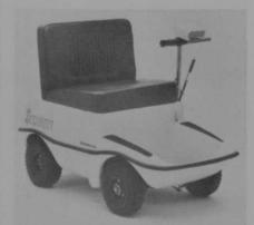
Auranthetic Corp. introduces the Mark 30, an electronically operated industrial vehicle. The new car features a transistorized-proportional speed control unit, forward and reverse, dynamic breaking and direct chain drive. The fiberglass car is chrome plated and has expanded vinyl seats. Two 12-volt batteries can propel the car for a distance of 30 miles at a maximum speed of 12 mph. Circle No. 106 on reader service card
