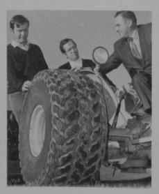
Firestone Tire & Rubber Company introduces the new Turf & Field rear tractor tire designed for golf courses, where damage to turf, particularly in sloping areas, has been a problem. The tire is 21 ½ inches wide with a low-profile design to provide traction while giving the floatation needed to prevent cutting and chunking of turf. The tire is designed for use on standard one-piece wheels. Circle No. 103 on reader service card
