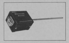
Vandermolen Corp. makes a soil moisture meter that registers when and how much to water different plants, turf, trees and crops. It will measure moisture content at any depth level up to 24 inches. The meter can be calibrated to compensate for mineral content in different soil Circle No. 108 on reader service card. types.
