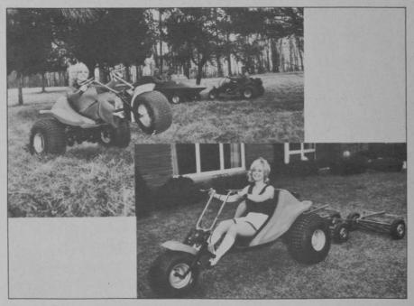
Alsport, Inc., announces a new high-performance three-wheel off road vehicle which can be used for high speed racing or for hitching up gang mowers, lawn rakes or utility carts. Only 34 inches high, the Tri-Sport is built to hug the ground at speeds up to 25 miles per hour. The Tri-Sport features a torque converter for automatic response, individual wheel control differential for light turns, band/drum brakes and low pressure tires.
