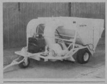
Vandermolen Corp. introduces the Diadem 290 spreader with a 50-foot cutting swath. It is capable of spreading fertilizer, seeds, herbicides, granular chemicals, salt or sand. It
