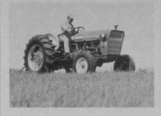
tures include an eight-speed transmission, wet disc brakes, three-point hitch, differential lock and power steering. Available with gas or diesel engines.
