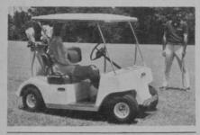
**Cushman Motors.**, Div. of Outboard Marine Corp. makes the *Trophy* four-wheel electric golf car, constructed of terneplate steel to resist corrosion. It features individual bucket seats, automotive steering and a 36-volt electric motor. A windshield and canopy are available.
