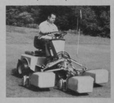
Hahn makes the *Tournament Triplex Greensmower* with precision cutting reels, variable speed control, hydrostatic drive and heavy-duty tee mowers, among other features.
