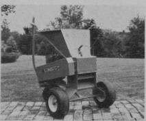
Chop-All Rotor which accepts a variety of material and chops it into one-half-inch sizes. Options include an attachment for leaf collection and a trailer. Also new is the SCM-720 Porta Screen with four bearing system suspension to prevent bogging down.
