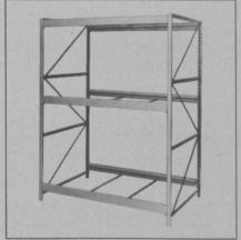
Lyon Metal Products, Inc., offers bulk storage racks for storing handloaded intermediate weight cartons. These racks have additional depth, width and height and are available in two, three and four-inch depths. Uprights range from five to 12 feet, beams are made of light, medium and heavy duty gauges in four, five and six and eight-foot lengths. Sections can stand alone or be joined.
