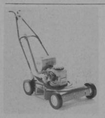
Goodall Div. has designed a heavy-duty, 22-inch, trim-type mower for commercial mowing. It comes with 8 by 1½ inch steel wheels with sealed ball-bearings and grease fittings that are recessed to permit close trimming, a hinged chute mulcher plate with a bracket to catch grass, heavy-gauge steel handles and a steel blade driver. The mower offers a choice of 3½ hp or 5hp engines with a 1½ quart extra oil base, five quart fuel tank and a snorket air cleaner mounted on the handle.
