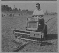
York Rakes Div. of York Modern Corp. offers a compact rake for use with garden tractors. The Model LFT is designed to remove thatch without damaging roots and clear away grass clippings, acorns and any other lawn debris. It uses three rotating tine bars with 117 spring teeth, each mounted on rubber. The rake clears a three foot swath, discharging material in neat rows. Available with a variety of hitches for attachment to garden tractors.
