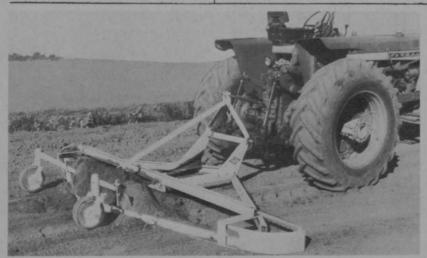
**DriAll Driers, Inc.**, introduces the LevLer, a low cost tool that eliminates ridges, depressions and furrows giving a smooth seed bed. The LevLer is equipped with a disc hitch for use behind a disc or three-point hitch. The LevLer comes in 11, 13, 15 and 17 foot models. Also available is a six-foot model for the compact trailer.
