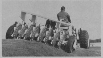
Here is a machine that really deep slices and conditions your contoured or hard turf. Exclusive design provides excellent low-contour following characteristics and in-line aerating for uniform penetration over uneven ground. Model 595 Aerator offers blade options which permit thatch removal and sub-turf aerating. Fits any tractor with 3-point or universal hitch. Operates at speeds up to 10 m.p.h.
