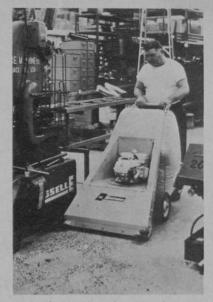
American Cleaning Equipment Corp. has designed the Compact 30 for indoor/outdoor vacuuming. It vacuums anything from sand and grit to broken glass and bulky debris. Among its other features are a 30-inch nozzle, heavy-duty filter bag and four hp gas or electric motor. The Compact 30 is 48 by 31 by 31 inches and is available with accessories.
