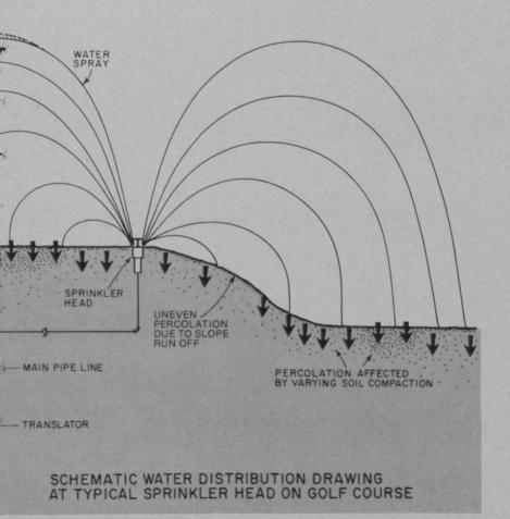
sprinkler systems. They can be cycled by central programming for chemical injection, but can also be scheduled with satellite controllers in the field that can be operated manually for on-the-spot supervision of chemical application. The running time of each head can actually be timed to adjust to the turf conditions of the area it covers.
