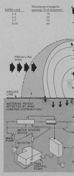
The number of heads required for effective watering goes up in inverse proportion to the square of spacing. Therefore, three times as many heads would be required in an eight to 10-mile-an-hour wind as are required in a zero to threemile-an-hour wind. Substantial savings may be effected simply by the operator scheduling watering periods to coincide with periods of day or night when winds are low.
