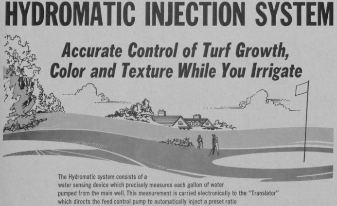
of fertilizer solution into the irrigation system in direct proportion to the water flow.
