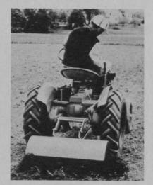
Engineering Products Company offers 32-inch rotary tiller for 12 and 14hp Economy tractors. Since there is no fluid-drive loss with Economy's 100 per cent geared drive-train, nearly all the tractor's 12 or 14hp can be applied to the tiller for fast, deep cutting.
