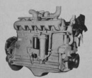
J I Case Company has developed a completely new family of four and six cylinder in-line, openchamber diesel engines for its construction, forestry and agricultural equipment. The engines range in power from 67 to 180 pto hp and Case plans to have them installed in almost every powered product in its entire line of equipment by early 1970.
