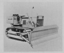
**J.I. Case Company** offers a dozer with a three-in-one hydraulically-controlled angling and tilting blade, which can be used as a straight dozer, a hydraulic angle dozer or as a hydraulic tilt dozer. While in motion, the blade may be turned as much as 20 degrees right or left and tilted up to 13 3/4 inches. According to the company, this is the only dozer in its class featuring total control of blade positioning from the operator's seat.
