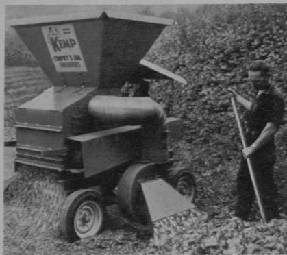
Kemp No. 7-0 with new, high-speed leaf handling vacuum blower attachment, shreds 20-30 cubic yards of soil an hour.
