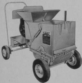
Kemp Model 8-0 (above) shreds 12 cu. yards of soil an hour. Other Kemp models range from 4 cu. yds. up to 101 cu. yds. an hour.
