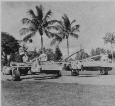
**Roseman Mower Corp.** has a new seven-gang Hydraulic Transport Mower, which features a new hitch design that, according to the company, permits greater flexibility. The mower can be used with any utility-type tractor equipped with a hydraulic system.
