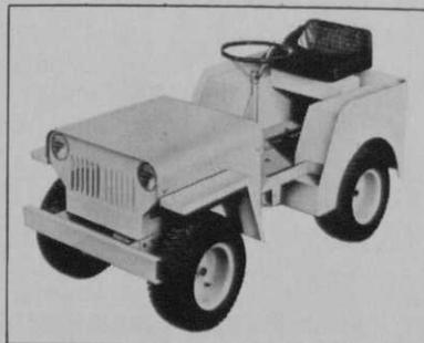
**C.F. Struck Corp.** has a compact lawn tractor called the Mini-Beeep. Available in a kit form, the four-wheel machine can be put together in less than three hours, according to the company. The kit, including a 7hp motor, is available for \$498.95.
