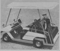
**Cushman Motors** manufacturers a three-way vehicle called the Town & Fairway. It features a two-passenger rear seat that pivots down to reveal two golf bag holders or the seat back can fold down to become a carry-all. Standard features on both electric and gasoline models include: surrey top, automotive steering, full front and rear suspension, headlights, taillights, turn signals and automatic seat brake.
