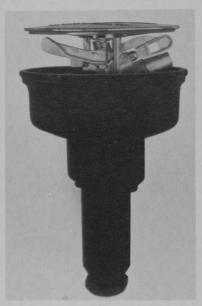
Febco, Inc., introduces a rotary popup sprinkler available in full or adjustable part circle models. Made of brass, the sprinkler is enclosed in a cast iron body with an aluminum cover and can be removed from the housing by unscrewing and lifting out. Both models have two parallel over-under nozzles and are impact driven by the top nozzle. Sprinklers operate in the 70 pound to 100 pound pressure range and cover up to a 256-foot circle.
