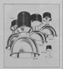
The Spero Electric Corp. markets a line of corrosion-resistant mercury vapor lighting fixtures. Called Balla Hi, the fixtures come equipped with sockets with stainless steel screw shells, special gaskets and spring pressure toggle latches. The line includes fixtures for 175, 250, 400 and 1,000-watt mercury vapor BT lamps and reflector lamps; they can also be made to accommodate metallic halide lamps.
