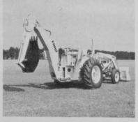
Ford Motor Company has increased by more than 11 per cent the loader-lift capacity of its Model 3400 tractor-backhoe-loader, according to the company. New features on this model include forward-thrusting front hood profile, manual reversing transmission, improved clutch life and comfort and convenience improvements for less operator fatigue. The model's 10-foot backhoe has a 10-foot, nine-inch, depth, a 14-foot-plus reach, and is available with Ford's "auto-dig" backhoe cycle.
