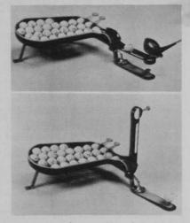
**IRA Products** introduces the Tee-Matic automatic golf ball teeing machine, which allows the golfer to tee up 30 consecutive golf balls without stooping. Made of heavy-gauge steel with baked on red and yellow enamel finish, the Tee-Matic retails for \$39.95.
